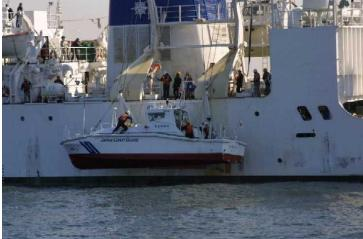
Jimbei is a small survey vessel. Through remote-control or previously programmed commands, it can survey bottom topographies and water temperatures unmanned.
