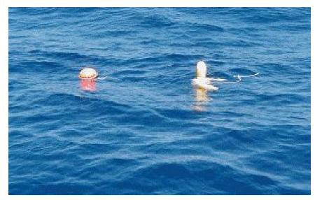
The Hydrographic Department, the 3rd Regional Headquarters of the Japan Coast Guard, located in Yokohama conducted an experiment of driftage on the sea surface using a manikin body model to trace its drifting path in Tokyo Wan (bay) in order to improve the prediction of driftage.
