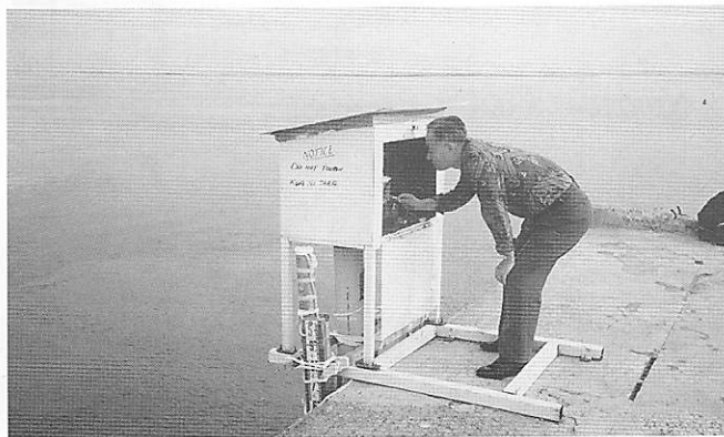
Tide station at Lakeba
