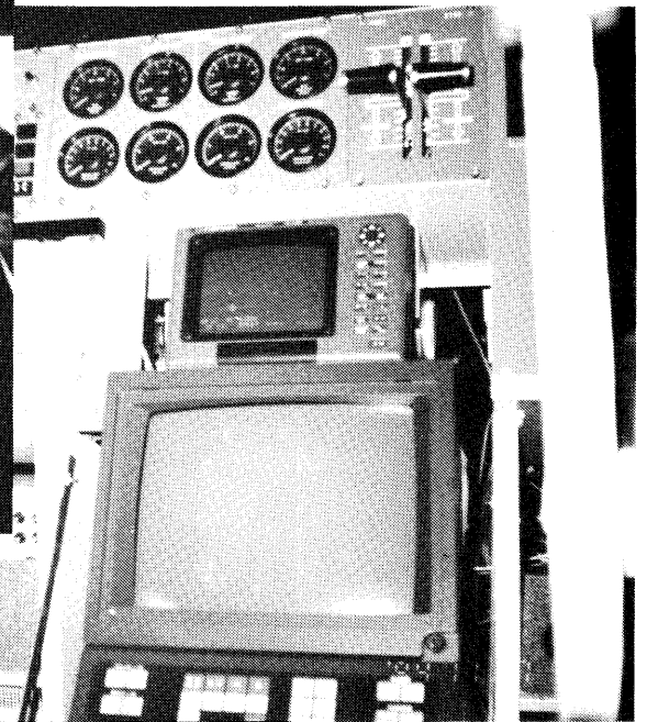
ERC system in the cockpit of the jetfoilship
