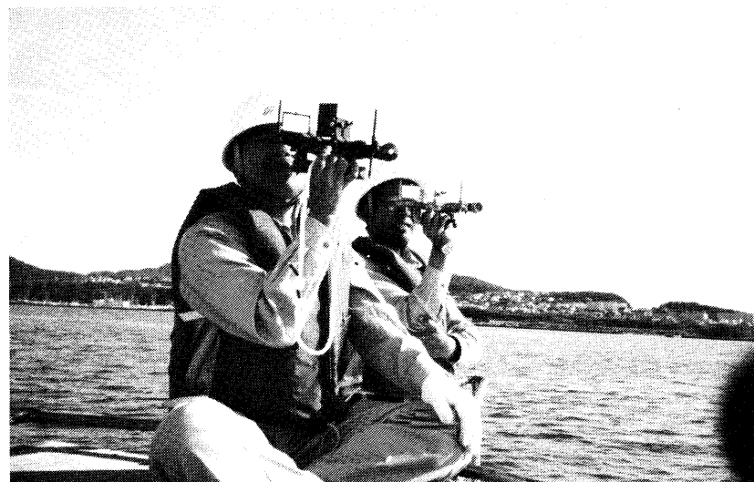
Practice on handling of a survey sextant on the survey launch
