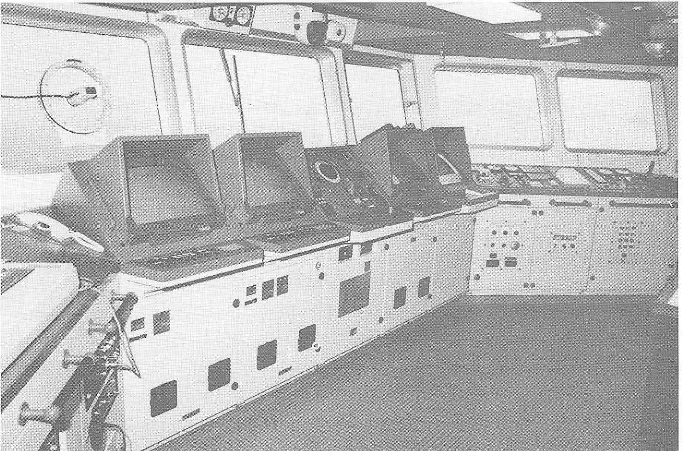
ERCS (two displays on the center of console) set in the total bridge system of a ship
